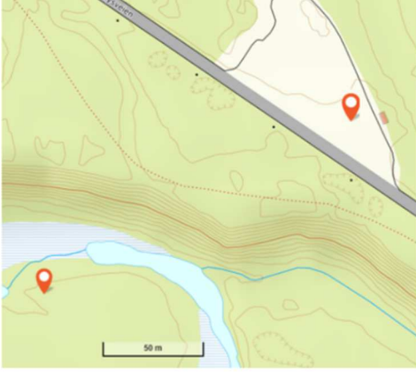
Fig. 3. Timeserver change of position during jamming represented on map. The signal degradation experienced by the timeserver during the jamming scenario caused the position reported by the timeserver to change by several hundred meters for as long as the interference persisted.
